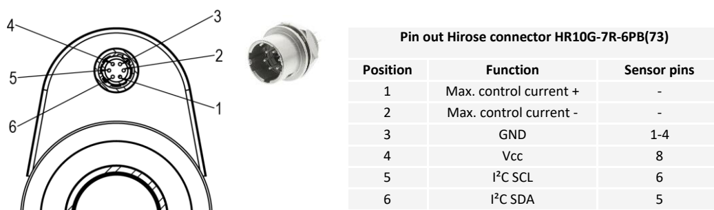
Figure 6: Electrical connections of lens models without embedded controller featuring (male) Hirose connector.
