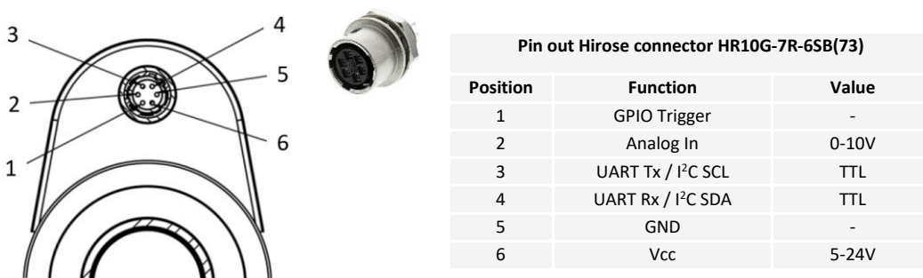
Figure 7: Electrical connections of lens models with embedded controller ECC-1C featuring (female) Hirose connector.
