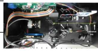
The internal iris may now be removed by unscrewing the iris from the rod.
