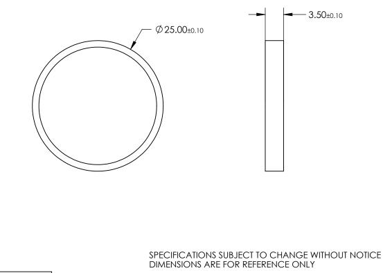
S1 S2 Edmund Optics® PLANO PLANO SHAPE 7 7 CONE HALF ANGLE (°) >5 OPTICAL DENSITY OD (AVERAGE) >5 700nm CWL, >OD5, 20nm FWHM Bandpass THIRD ANGLE 80 - 50 TITLE 80 - 50 SURFACE QUALITY Filter, 25mm Dia. ≥Ø10.00 ≥Ø10.10 CLEAR APERTURE SHEET DWG NO ALL DIMS IN mm PROTECTED AS NEEDED PROTECTED AS NEEDED 78446 BEVEL 37 OF 52
