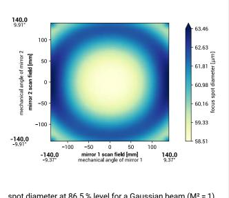
spot diameter at 86.5% level for a Gaussian beam (M² = 1) with 14.0 mm diameter at  $1/e^2$ , clipped at 14.0 mm field size and mirror distances as given above for a two mirror scan system
