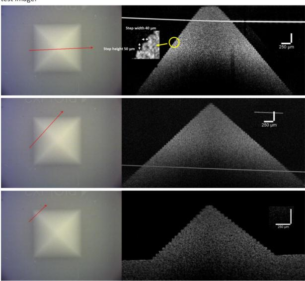
OCT test system specifications: Spectral Domain OCT Imaging System, 1300 nm, axial resolution is 5.5 microns, lateral resolution of 13 microns.
