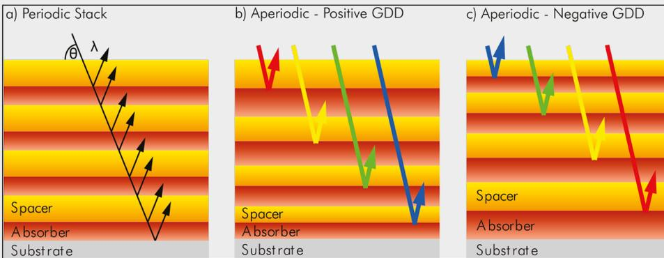
Different multilayer stack designs. a) Physical principle of a XUV/soft X-ray multilayer mirror for a periodic design (nearly gaussian reflectivity and chirp free spectral phase). Phase corrections can be realized with aperiodic designs introducing a (b) positive or (c) negative group delay dispersion (GDD).
