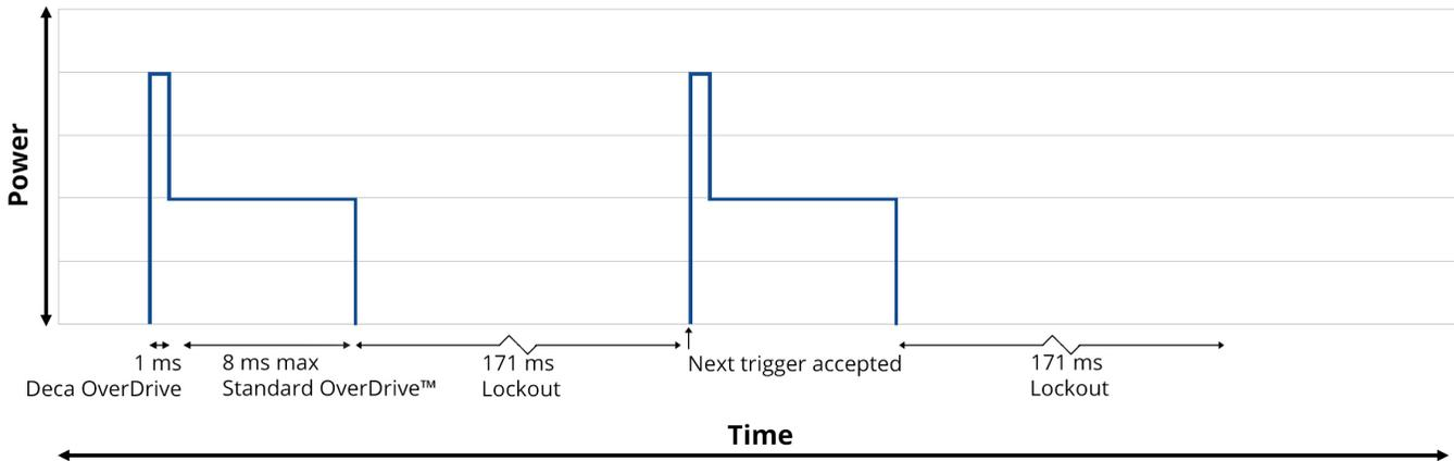
The duty cycle of Dual OverDrive on the JWL225-DO Series is 5%.
