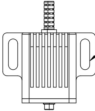
MOUNTING SLOTS COMPATIBLE WITH BREADBOARDS WITH 50mm OR 2in HOLE SPACING
