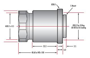
Figure 3. External schematic of a Cw Series Lens.
