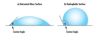
Figure 2. Two water droplets on horizontal glass surface. a) There is a smaller contact angle on the untreated surface, indicating higher surface tension. b) There is a larger contact angle on the hydrophobic surface, indicating lower surface tension.
