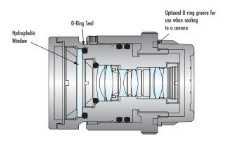
Figure 1. Internal schematic of a Cw Series Lens.
