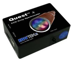
The Quest<sup>TM</sup> X is a linear CCD array spectrometer optimized for UV and NIR performance using a low stray light optical bench. It features a 2048 element detector, built-in 16-bit digitizer, USB 2.0 interface with a >2.0 MHz readout speed, and external trigger. The Quest<sup>TM</sup> X is temperature compensated, which greatly reduces the thermal drift to ~15 counts/°C. This gives improved stability by decreasing baseline drift and sustaining the dynamic range.
