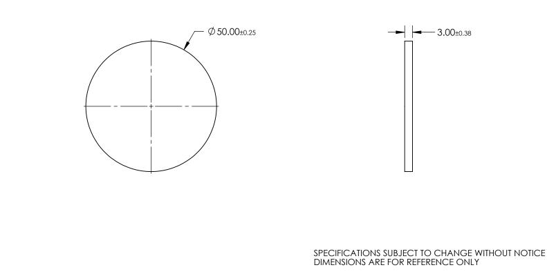
Edmund Optics® S1 PLANO SHAPE HEAT ABSORBING FUNCTION ISUZU ISK153, 50 Dia., HEAT ABSORBING THIRD ANGLE TITLE 60-40 SURFACE QUALITY COLORED GLASS FILTER Ø45.00 CLEAR APERTURE SHEET ALL DIMS IN DWG NO mm PROTECTIVE AS NEEDED 15710 BEVEL MAX FACE 1 OF 1
