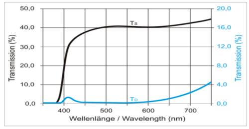
The CP42HE circular polarizer is created by laminating the XP42 linear polarizer to the high contrast WP140HE ¼ wavelength retarder sheet. The process results in one of the best circular polarizers available on the market, offering the highest contrast and maximum light transmission for the most demanding of applications.
