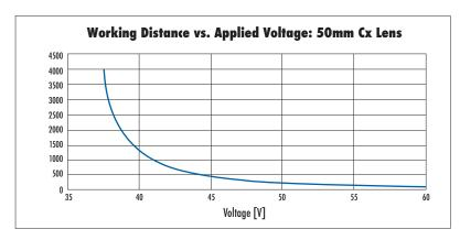
Figure 5: Working distance as a function of voltage applied to liquid lens for 50mm Cx Lens.
