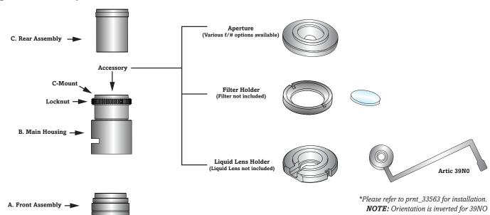
Warning: Liquid Lens ribbon is fragile. Use caution when assembling unit and during handling.
