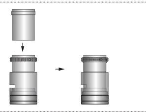
4. Adjust Locknut position until desired focus is achieved. See section on Working Distance and Field of View below to find Locknut positions. Tighten Nylon Tip Set Screw into place for a focal position that can later be readjusted—the nylon tip will protect the threads. To set focal position permanently, install the socket head screws. Do not overtighten screws.
