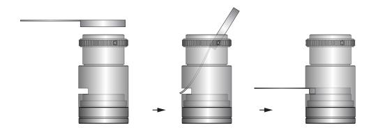
3. Using a spanner wrench, thread the bottom of Rear Assembly into the top of Main Housing until it is flat against the accessory, hand tightening torque or about 2.5-5kgf\*cm. If using a Liquid Lens, hold the Liquid Lens in place while tightening the Rear Assembly into Main Housing by inserting a paper-clip into one of the holes to the side of the Liquid Lens Holder. (Optional: spanner wrench #35-029 can be used)
