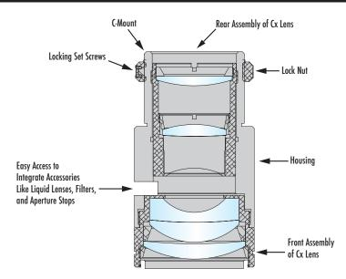
Figure 1: 50mm Cx lens without the required accessory.
