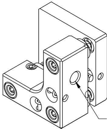
M4 x 0.7 x 7 DEEP FOR MOUNTING THE KINEMATIC ASSEMBLY (2X)
