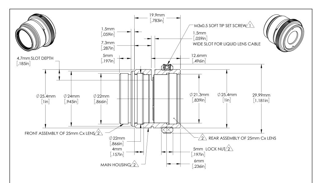
1.\ 3 m3x0.5 flat point stainless steel set screws included to optionally FIT 3 HOLES IN LOCK NUT, 120° APART.
