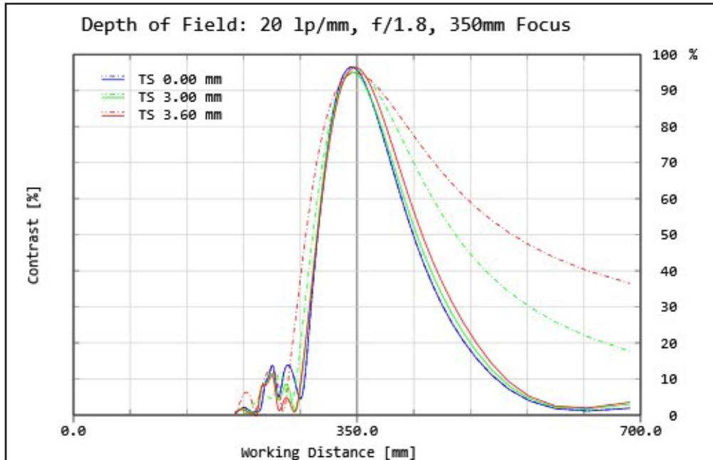
**Figure 6:** Polychromatic diffraction through-focus MTF at 20 linepairs/mm (image space). Contrast is plotted to two times the focus distance. Note object spatial frequency changes with working distance.
