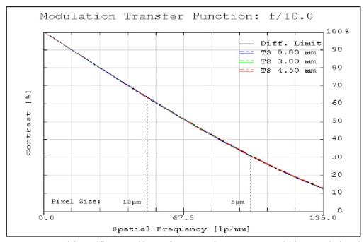
Figure 5: Image space polychromatic diffraction FFT Modulation Transfer Function (MTF) for  $\lambda = 486$ nm to 656nm. Included are Tangential and Sagittal values for field points on center, at 70% of full field and at the maximum sensor format. Solid black line indicates diffraction limit determined by f/#-defined aperture. Frequencies corresponding to the Nyquist resolution limit of pixel sizes are indicated.
