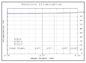
Figure 2: Relative illumination (center to corner)
