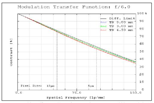
Figure 3: Image space polychromatic diffraction FFT Modulation Transfer Function (MTF) for  $\lambda = 486$ nm to 656nm. Included are Tangential and Sagittal values for field points on center, at 70% of full field and at the maximum sensor format. Solid black line indicates diffraction limit determined by f/#-defined aperture. Frequencies corresponding to the Nyquist resolution limit of pixel sizes are indicated.
