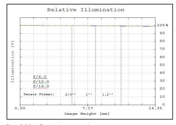
Figure 2: Relative illumination (center to corner)
