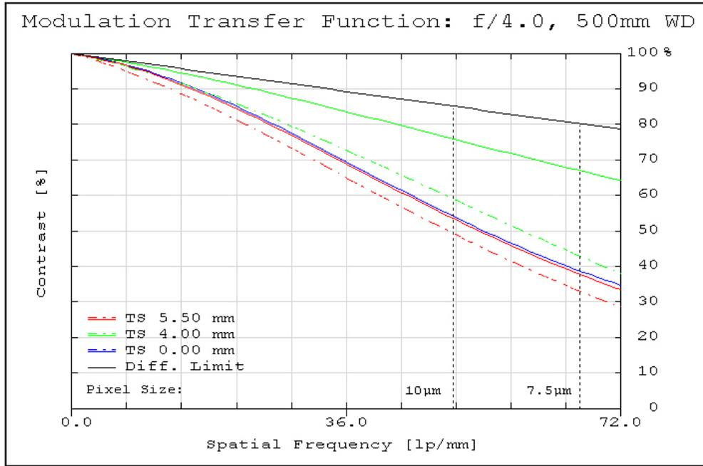
**Figure 5:** Image space polychromatic diffraction FFT Modulation Transfer Function (MTF) for  $\lambda = 486\text{nm}$  to  $656\text{nm}$ . Included are Tangential and Sagittal values for field points on center, at 70% of full field and at the maximum sensor format. Solid black line indicates diffraction limit determined by  $f/\#$ -defined aperture. Frequencies corresponding to the Nyquist resolution limit of pixel sizes are indicated.
