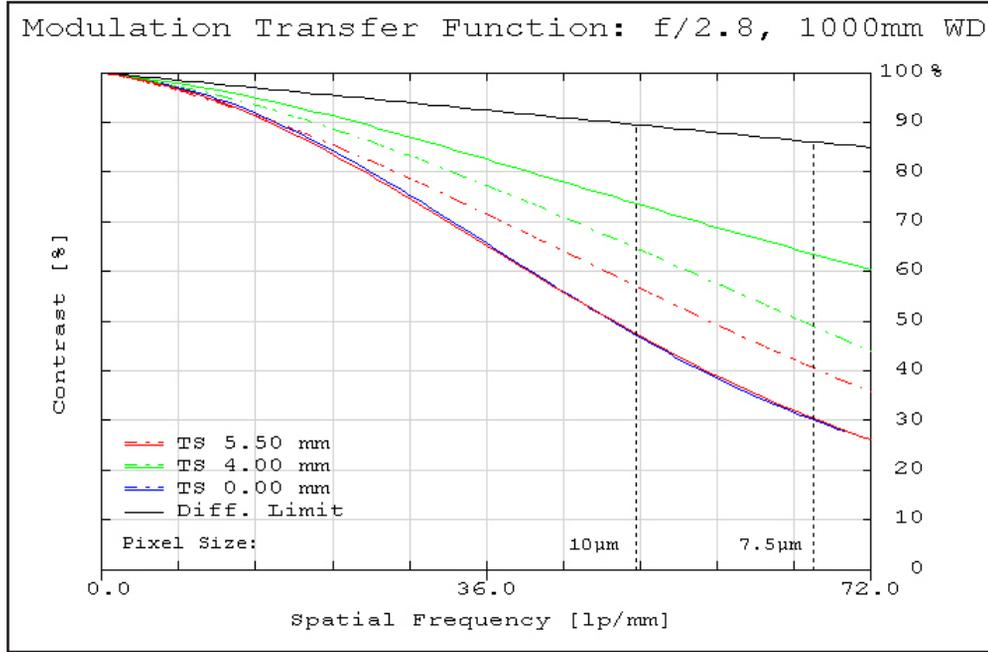
**Figure 7:** Image space polychromatic diffraction FFT Modulation Transfer Function (MTF) for  $\lambda = 486\text{nm}$  to  $656\text{nm}$ . Included are Tangential and Sagittal values for field points on center, at 70% of full field and at the maximum sensor format. Solid black line indicates diffraction limit determined by  $f/\#$ -defined aperture. Frequencies corresponding to the Nyquist resolution limit of pixel sizes are indicated.
