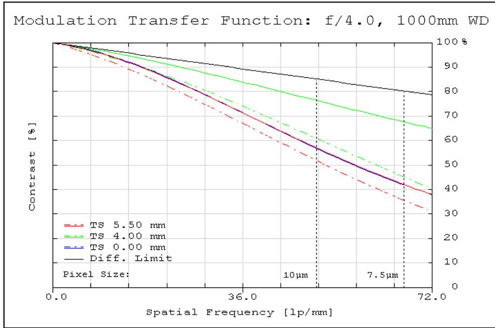
**Figure 9:** Image space polychromatic diffraction FFT Modulation Transfer Function (MTF) for  $\lambda = 486\text{nm}$  to  $656\text{nm}$ . Included are Tangential and Sagittal values for field points on center, at 70% of full field and at the maximum sensor format. Solid black line indicates diffraction limit determined by  $f/\#$ -defined aperture. Frequencies corresponding to the Nyquist resolution limit of pixel sizes are indicated.
