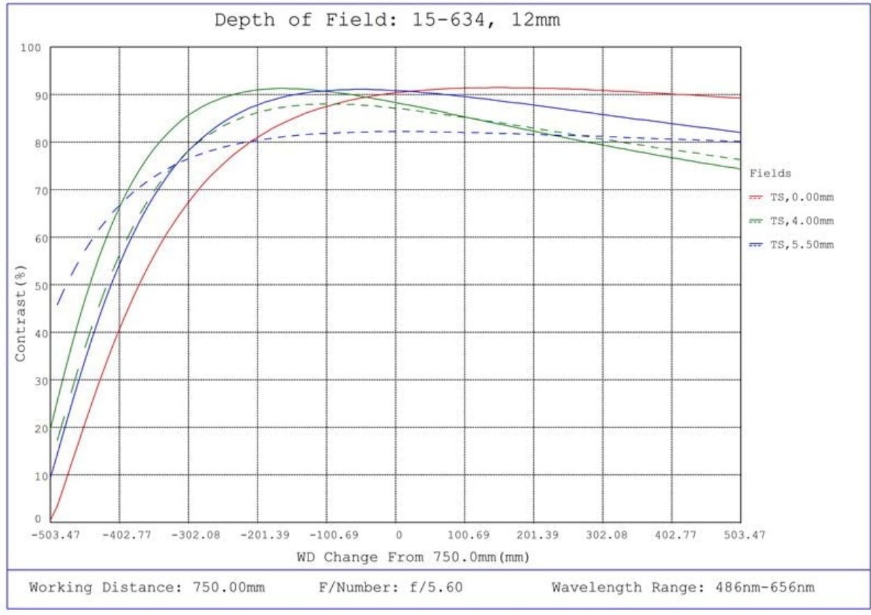
#15-634, 12mm, f/5.6 Cw Series Fixed Focal Length Lens, Depth of Field Plot, 750mm Working Distance, f5.6
