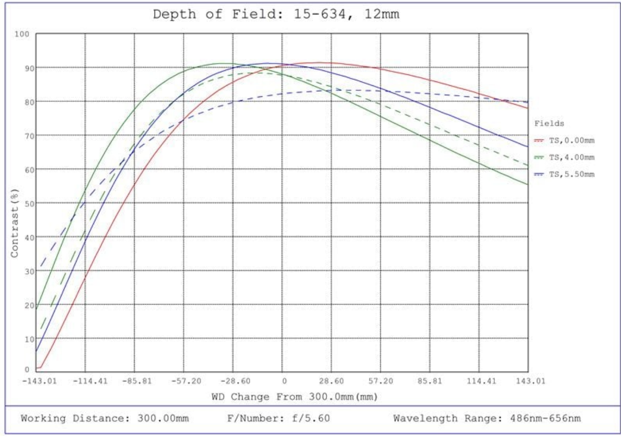
#15-634, 12mm, f/5.6 Cw Series Fixed Focal Length Lens, Depth of Field Plot, 300mm Working Distance, f5.6
