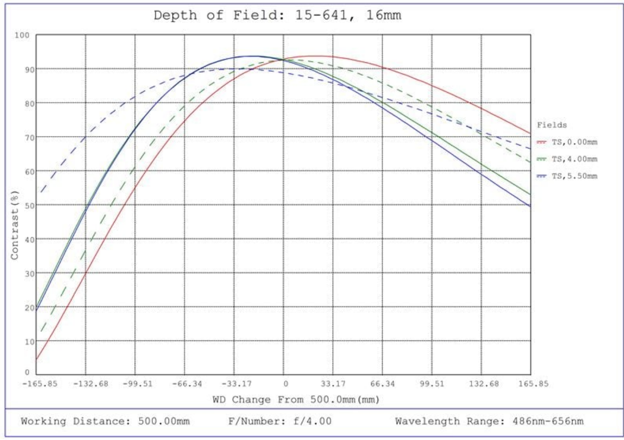
#15-641, 16mm, f/4 Cw Series Fixed Focal Length Lens, Depth of Field Plot, 500mm Working Distance, f4
