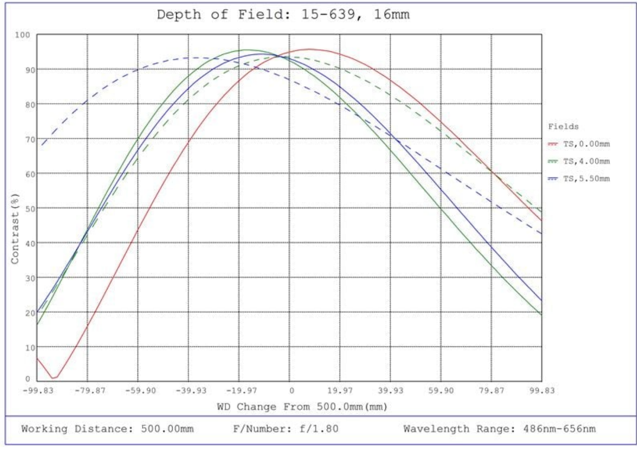
#15-639, 16mm, f/1.8 Cw Series Fixed Focal Length Lens, Depth of Field Plot, 500mm Working Distance, f1.8
