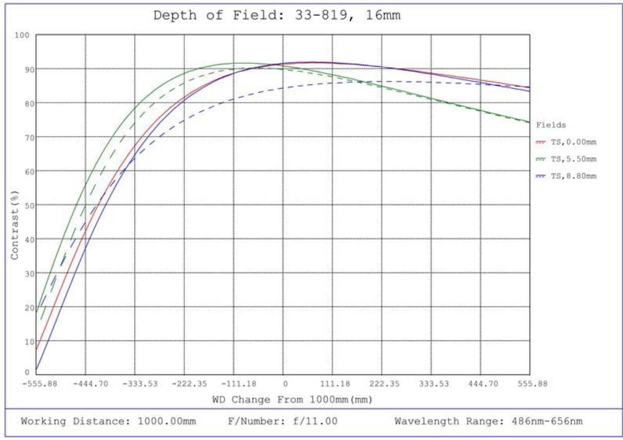
#33-819, 16mm f/11, HPi Series Fixed Focal Length Lens, Depth of Field Plot, 1000mm Working Distance, f11
