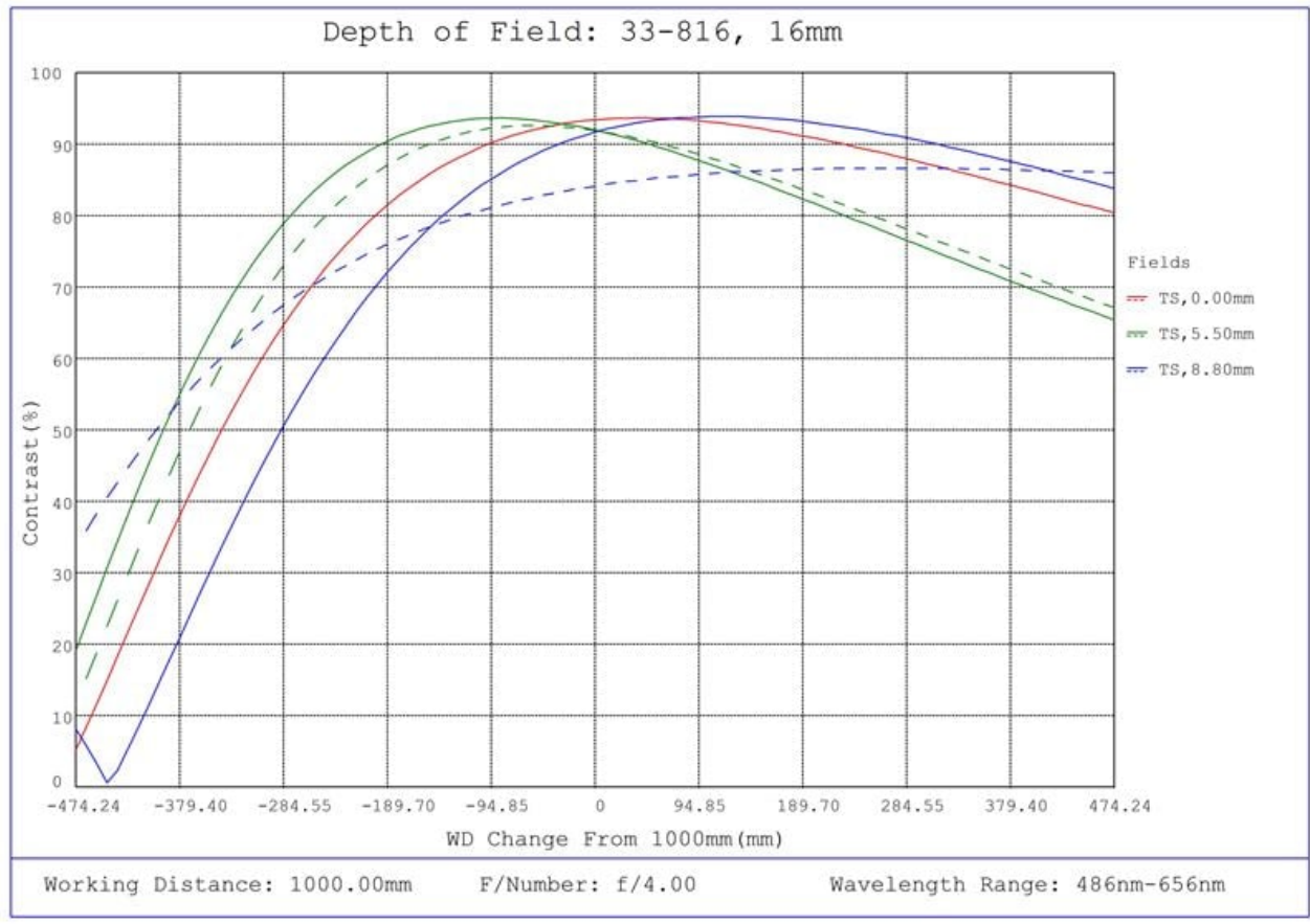
#33-816, 16mm f/4, HPi Series Fixed Focal Length Lens, Depth of Field Plot, 1000mm Working Distance, f4
