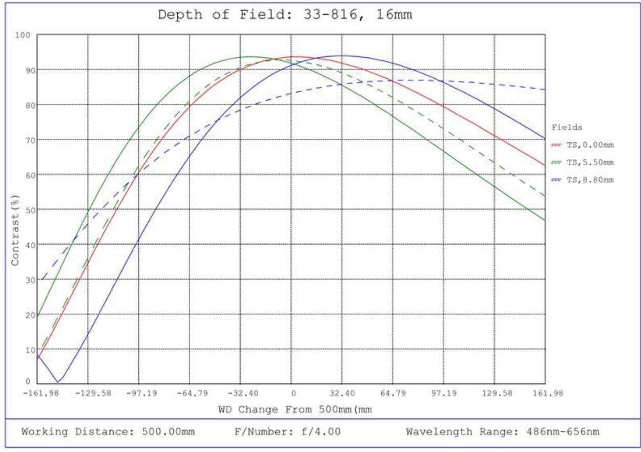
#33-816, 16mm f/4, HPi Series Fixed Focal Length Lens, Depth of Field Plot, 500mm Working Distance, f4
