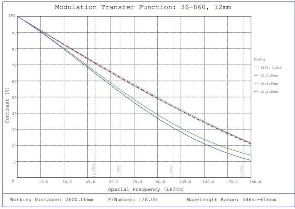
#36-860, 12mm f/8, 1000mm-∞ Primary WD, HRr Series Fixed Focal Length Lens, Modulated Transfer Function (MTF) Plot, 2600mm Working Distance, f8
