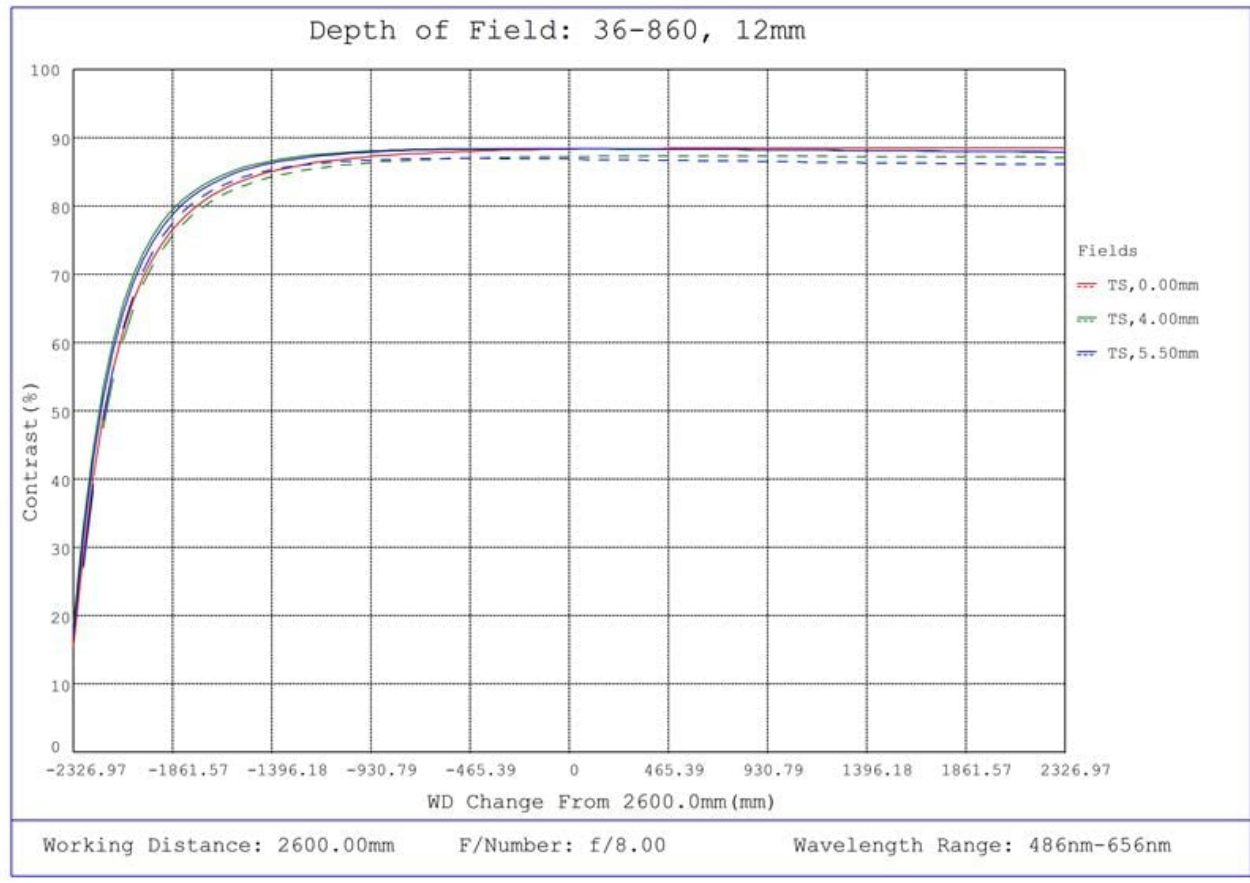
#36-860, 12mm f/8, 1000mm-∞ Primary WD, HRr Series Fixed Focal Length Lens, Depth of Field Plot, 2600mm Working Distance, f8
