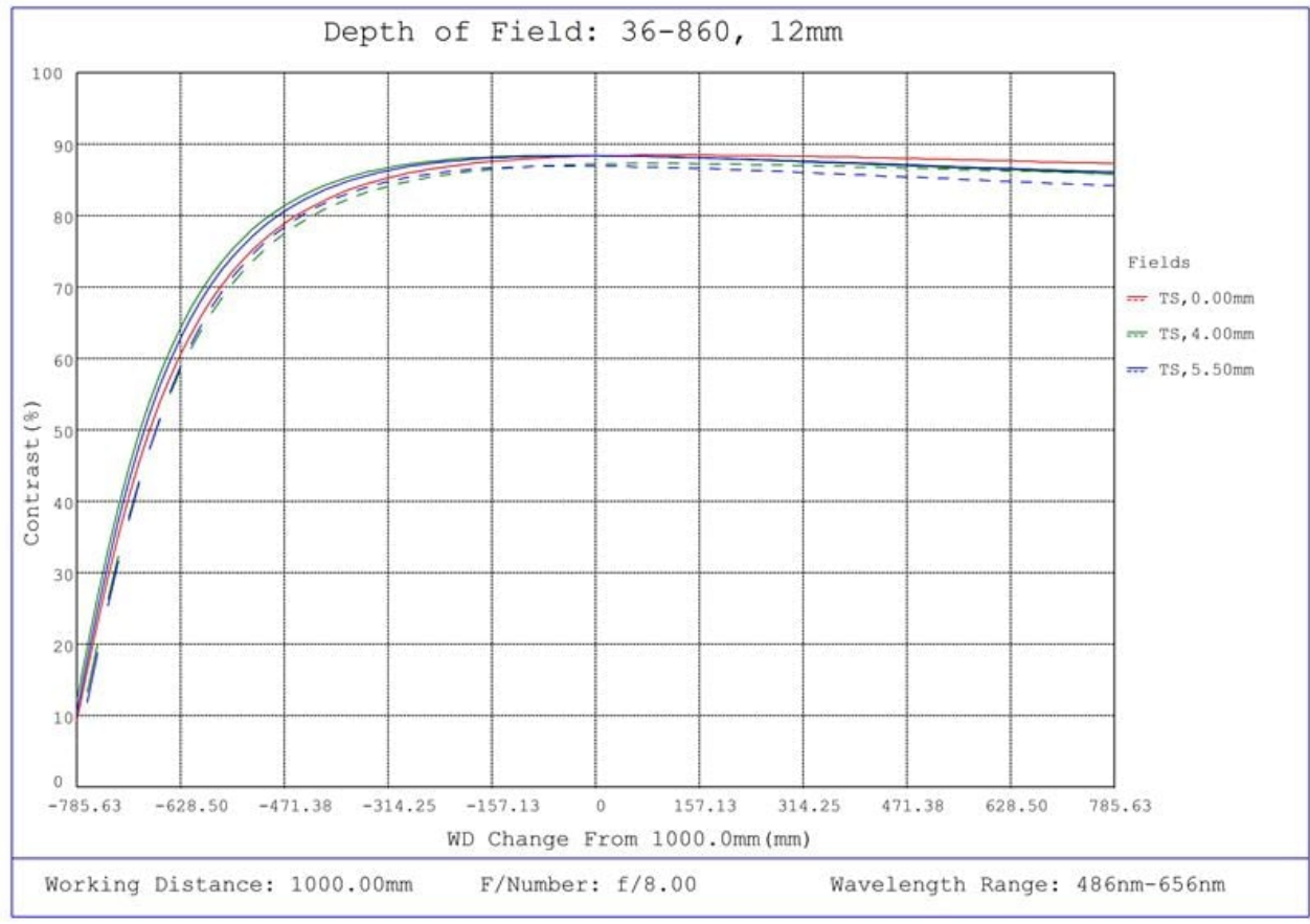
#36-860, 12mm f/8, 1000mm-∞ Primary WD, HRr Series Fixed Focal Length Lens, Depth of Field Plot, 1000mm Working Distance, f8
