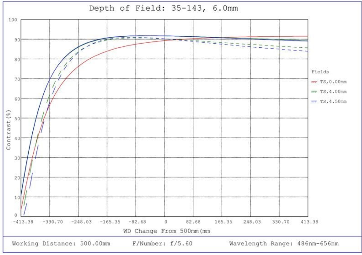
#35-143, 6mm, f/5.6 Cr Series Fixed Focal Length Lens, Depth of Field Plot, 500mm Working Distance, f5.6
