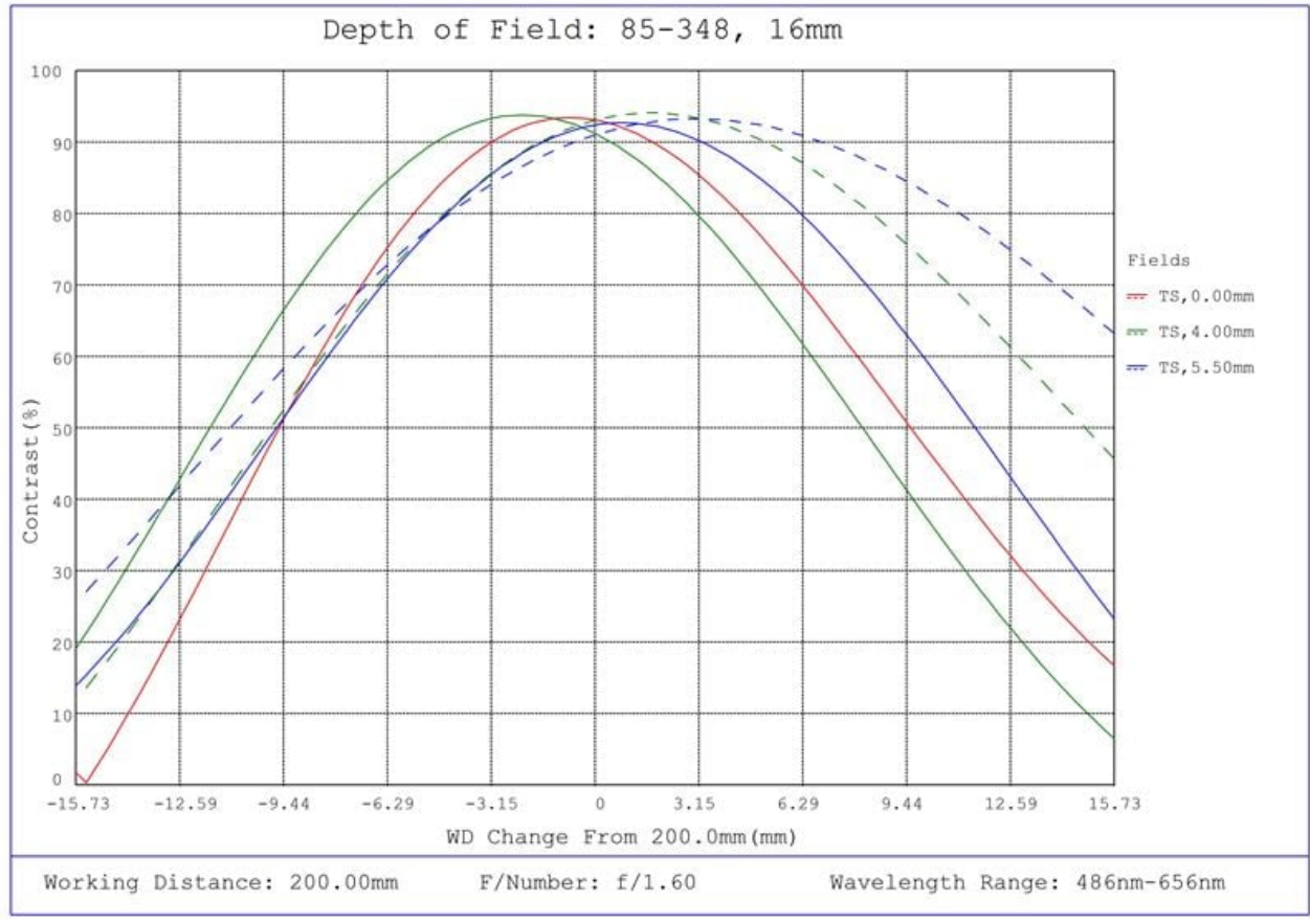
#85-348, 16mm, f/1.6 Ci Series Fixed Focal Length Lens, Depth of Field Plot, 200mm Working Distance, f1.6
