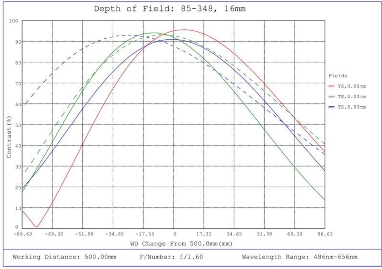
#85-348, 16mm, f/1.6 Ci Series Fixed Focal Length Lens, Depth of Field Plot, 500mm Working Distance, f1.6
