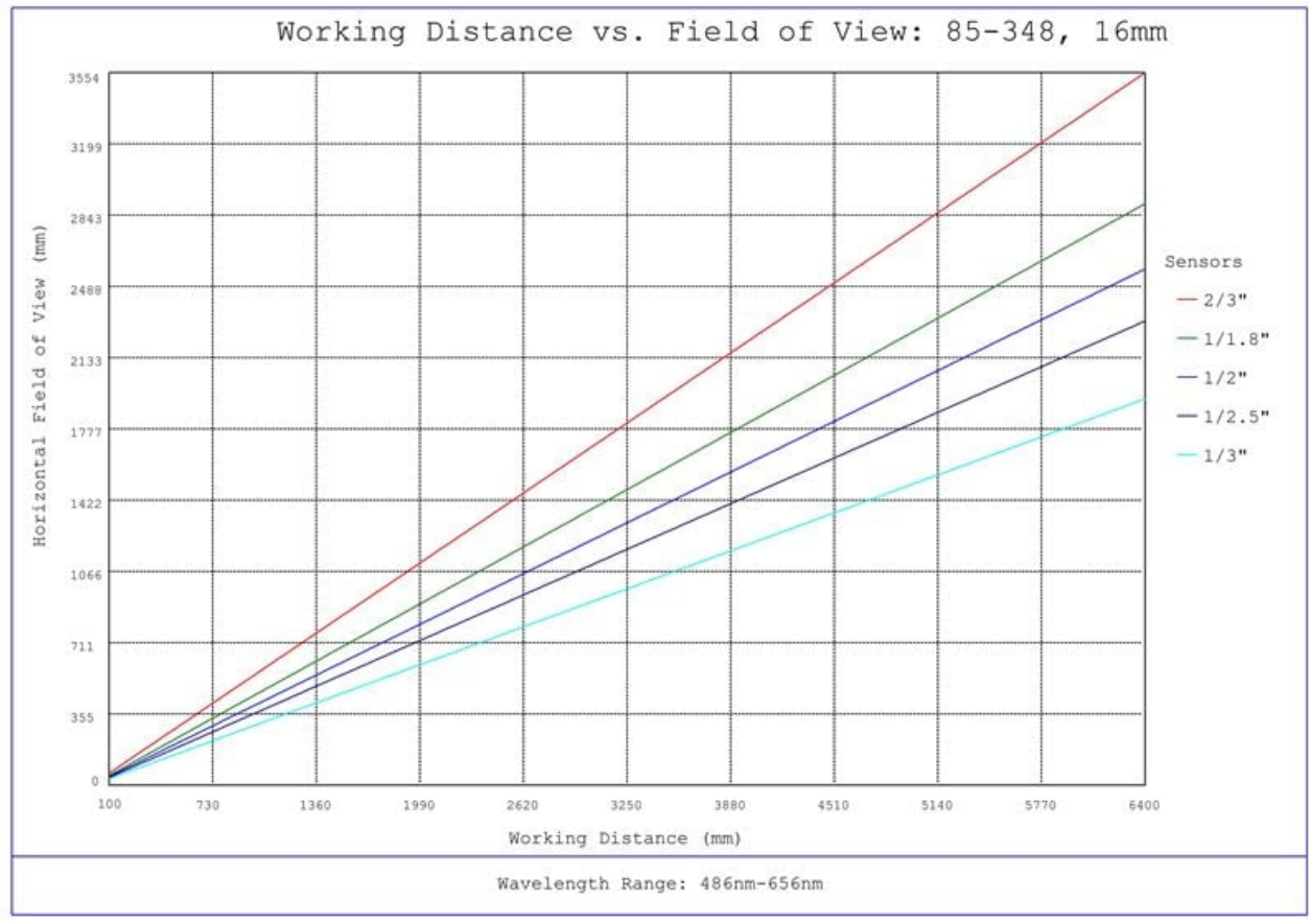
#85-348, 16mm, f/1.6 Ci Series Fixed Focal Length Lens, Working Distance versus Field of View Plot
